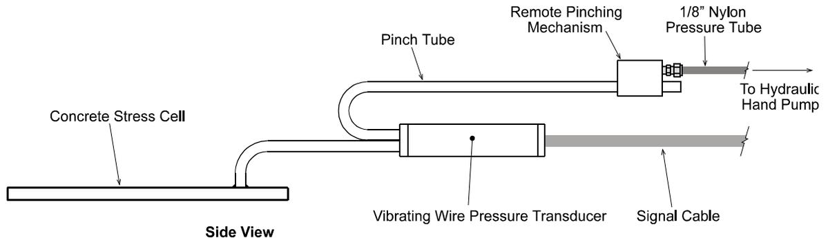
Figure 7 - Model 4850 with Remote Pinching Apparatus
