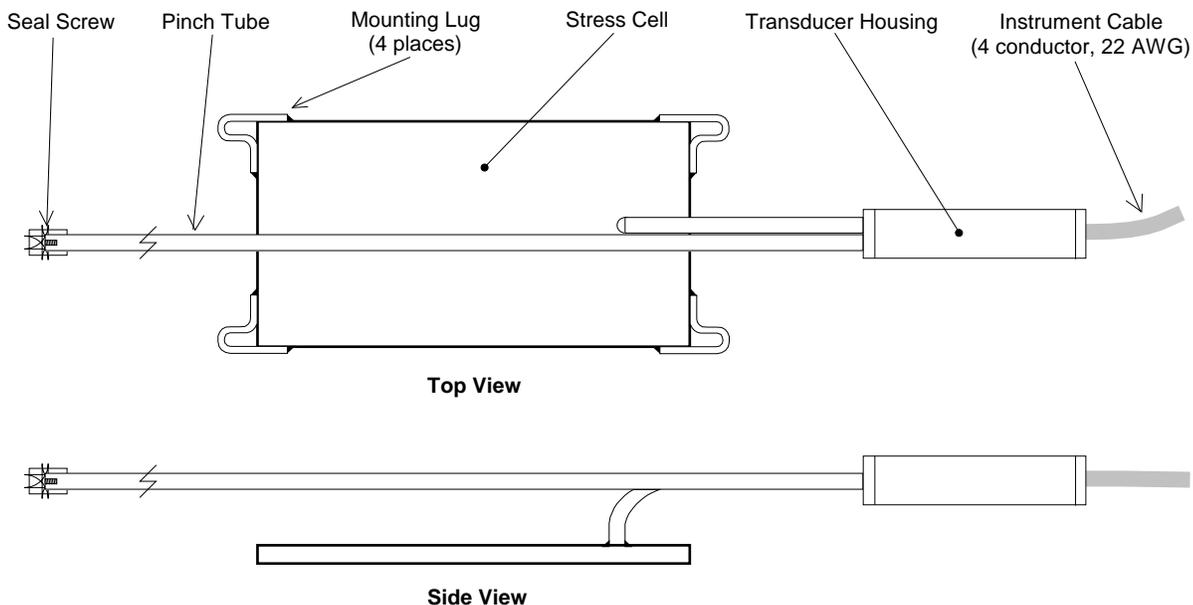
Figure 2 - Model 4850 Concrete Stress Cell
