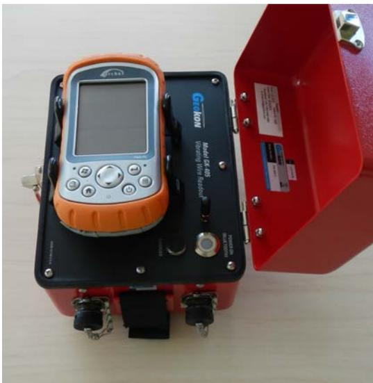
Figure 8 GK405 Readout Unit
