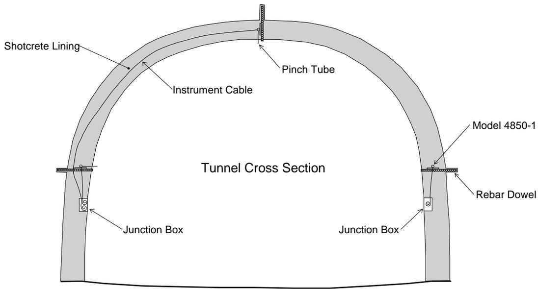
**Figure 3 - Model 4850-1 Installation**
