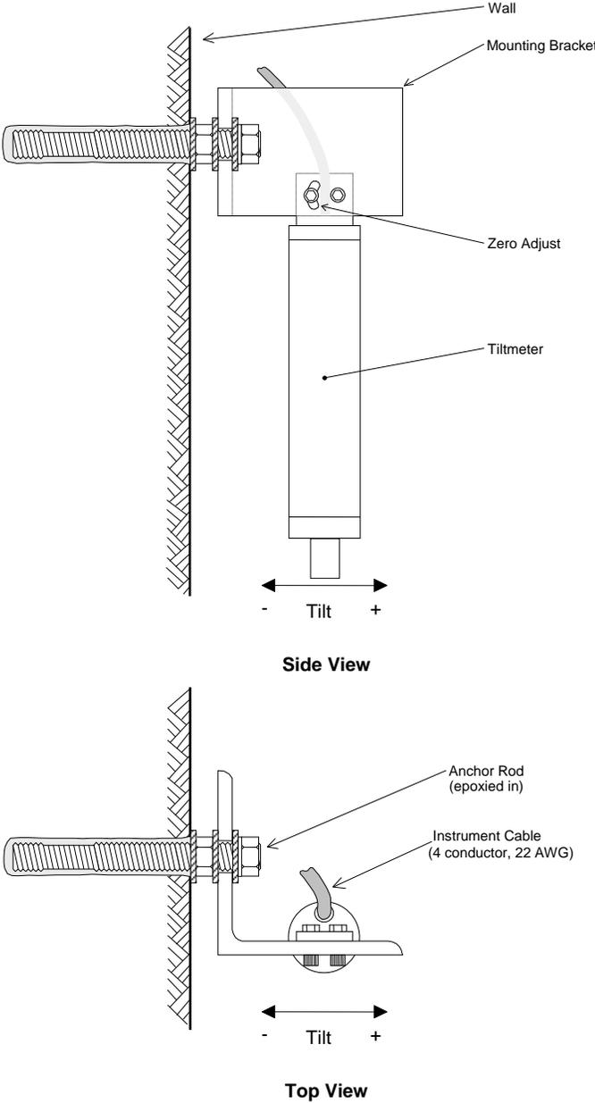
Figure 1 - Model 6350 Uniaxial Tiltmeter Installation
