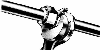
3 The connection can now be made by following the Re-tightening Instructions.
