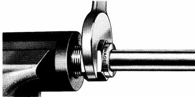
Assemble SWAGELOK nut and ferrules to pre-swaging tool. Insert tubing through ferrules until it bottoms in the pre-swaging tool, and tighten nut 1-1/4 turns.\*
