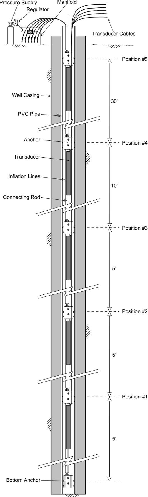
Figure 2 - Model A-9 Installation
