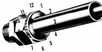
Before tightening the SWAGELOK nut, scribe the nut at the 6 o'clock position.
