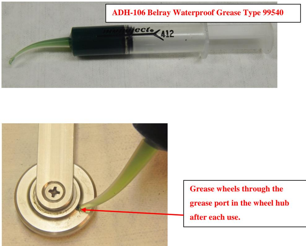
Figure 4. Wheel Lubrication
