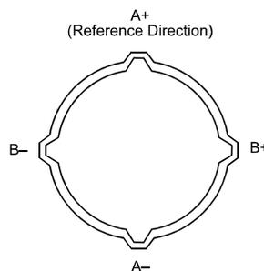
Figure 3 Inclinometer Casing
