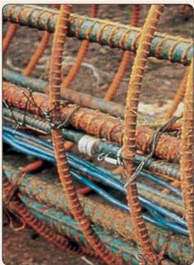
• Close-up of Model 3911 shown as installed in concrete pile reinforcing cage.
