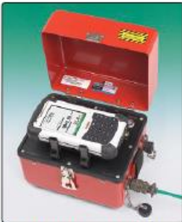
• Geokon Model GK-405 WW Readout for use with the Model 4000 and 4050 Strain Gages.
