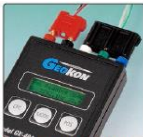
• Closeup of the Model GK-404 with banana-jack connections.
