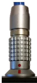
Figure 9 - Lemo Connector to GK-404
