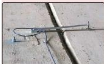
• Model 4420-3 Low Profile Crackmeter for measurements in the "Z" direction.
