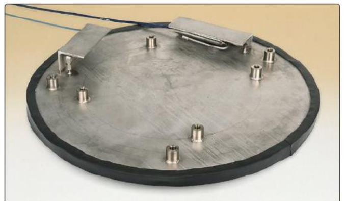
● Model 4855 Pile Tip Pressure Cell.
