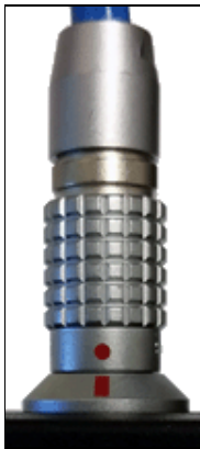
FIGURE 17: Lemo Connector to GK-404
