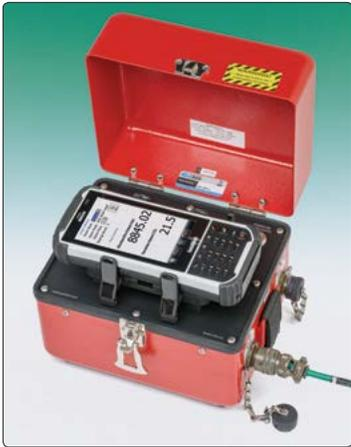
● Model GK-405 Vibrating Wire Readout for manual data acquisition.
