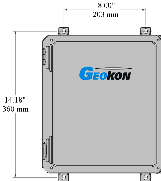
Figure 9 - Multiplexer Enclosure Mounting Dimensions
