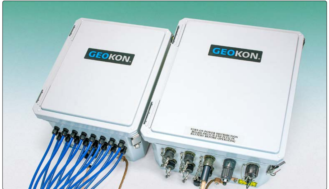
• Model 8600-1 Datalogger (right) and the Model 8032 16 Channel Multiplexer (left).
